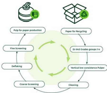
Figure 1. Recycling in standard paper mills.
